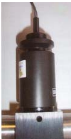
the aspirated adaptor on probe for fixed location monitoring
